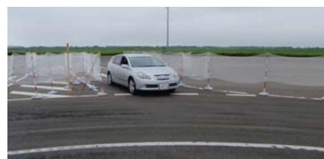
Simulated snow piles and Test vehicle
